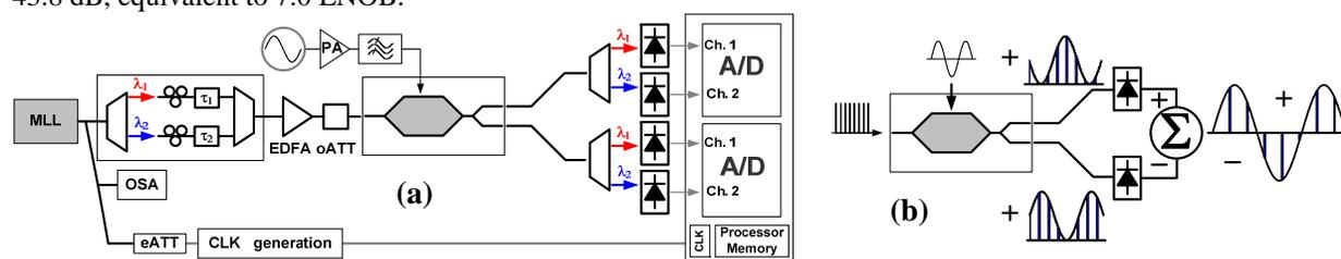
Figure 1 (a) The schematic of the testbed. (b) The balanced detection scheme that creates bipolar output, improving SNR by 6 dB.
