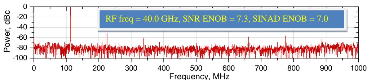
Figure 2 RF spectrum of the subsampled 40 GHz input tone at the rate of 2 GSa/s.
