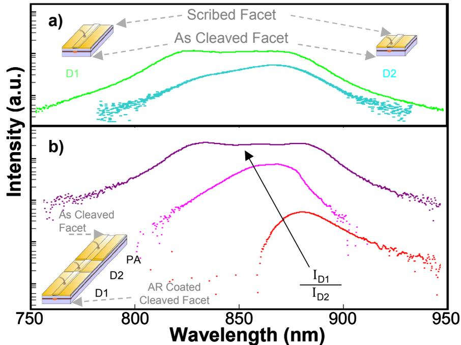
Fig. 6. The measured spectra from (a) a stand-alone gain section with scribed facets at a current injection of 200 mA and (b) three-section SLD with AR coating with varying current ratio of  $D_1$  (500  $\mu\text{m}$ ) to  $D_2$ .
