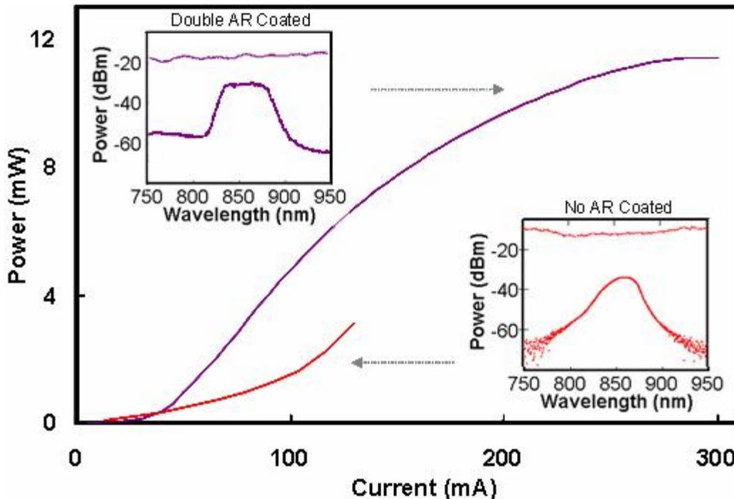
Fig. 7. The optical power versus total injection current to  $D_1$  section ( $850 \mu\text{m}$ ) of the three-section SLD with and without AR coating (on the emitter and absorber facet). The inset shows the corresponding spectrum and modulation for both
