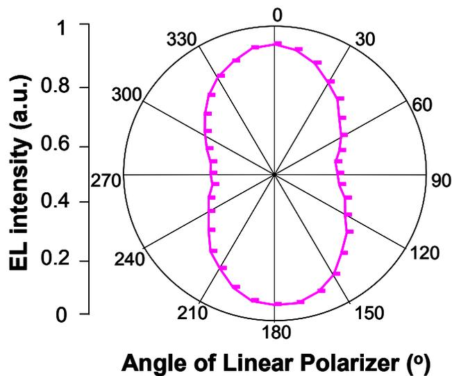
Fig. 2. Normalized optical power at various angle of rotation of a polarizer. The emission is thus characterized as being elliptically polarized TE/TM 2:1.
