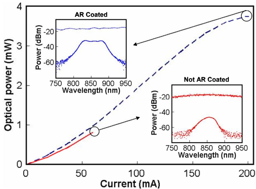
Fig. 3. The optical power versus total injection current to the  $D_1$  section (500  $\mu\text{m}$ ) of the three-section SLD with and without AR coating on the emitter facet. The inset shows the corresponding spectrum and modulation for both devices measured using a spectrum analyzer with a resolution of 2 nm and 0.05 nm respectively.
