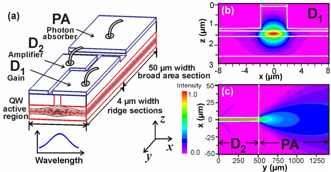
Fig. 1. (a) The schematic device structure of three-section QW SLD consisting of two 4 μm wide ridge waveguide active sections (D<sub>1</sub> and D<sub>2</sub>) and an integrated 50 μm wide broad area photon absorber (PA). (b) The simulated cross section of the optical confinement in the ridge waveguide D<sub>1</sub> and D<sub>2</sub>. (c) The simulated light spreading along the longitudinal direction y from D<sub>2</sub> to PA.
