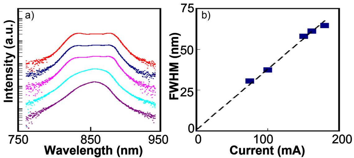
Fig. 4. a) Optical spectra acquired with a spectrum analyzer resolution of 2 nm for various injected currents to the  $D_1$  section (which is 500  $\mu\text{m}$  in length and AR coated) of the three-section SLD. b) The corresponding FWHM of an SLD with increasing injection current.
