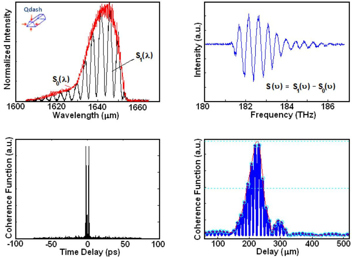
Figure 6. Measured QD BLD source spectrum,  $S_0(\lambda)$ , and corresponding spectral interferogram,  $S_I(\lambda)$ , as well as the calculated  $S(\nu)$  and coherence function in terms of time and distance delay.
