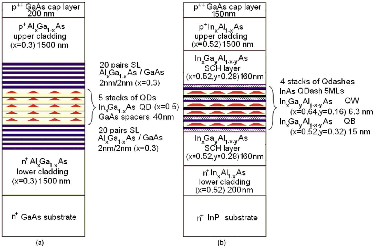
Figure 3. The InGaAs/GaAs QD (a) and the InAs/InAlGaAs Qdash (b) wafer structure composition.
