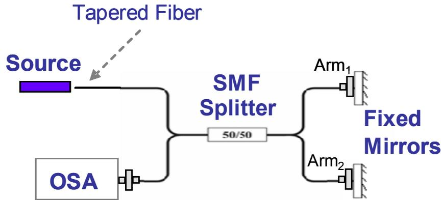
Figure 1. The schematic of fiber-based spectral interferometric system used in our experiment. This system consists of a broadband light source (either a SLD or BLD) coupled into a tapered SMF, a 2x2 fiber splitter/combiner, Arm<sub>1</sub> and Arm<sub>2</sub> that are in contact with fixed Au-coated mirrors, and an OSA for signal detection.
