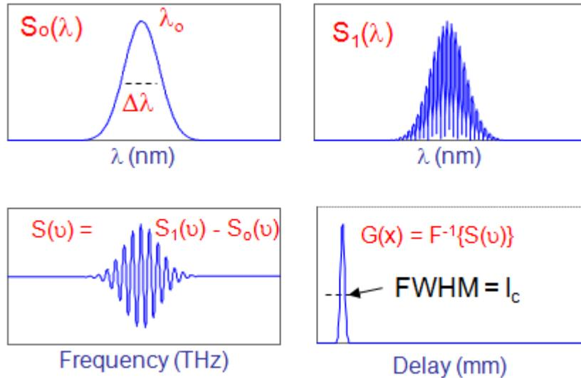
Figure 2. Ideal Gaussian simulated functions for the input,  $S_0(\lambda)$ , and the corresponding spectral interferogram,  $S_1(\lambda)$ , as well as  $S(v)$ , which is  $S_1(v) - S_0(v)$  and  $G(x)$ , the coherence function.
