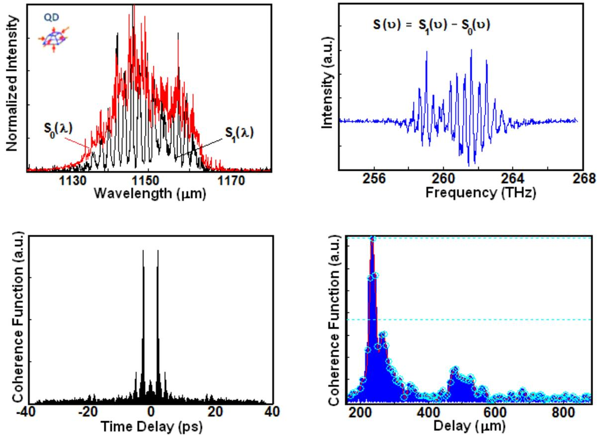
Figure 5. Measured QD BLD source spectrum,  $S_0(\lambda)$ , and corresponding spectral interferogram,  $S_I(\lambda)$ , as well as the calculated  $S(\nu)$  and coherence function in terms of time and distance delay.
