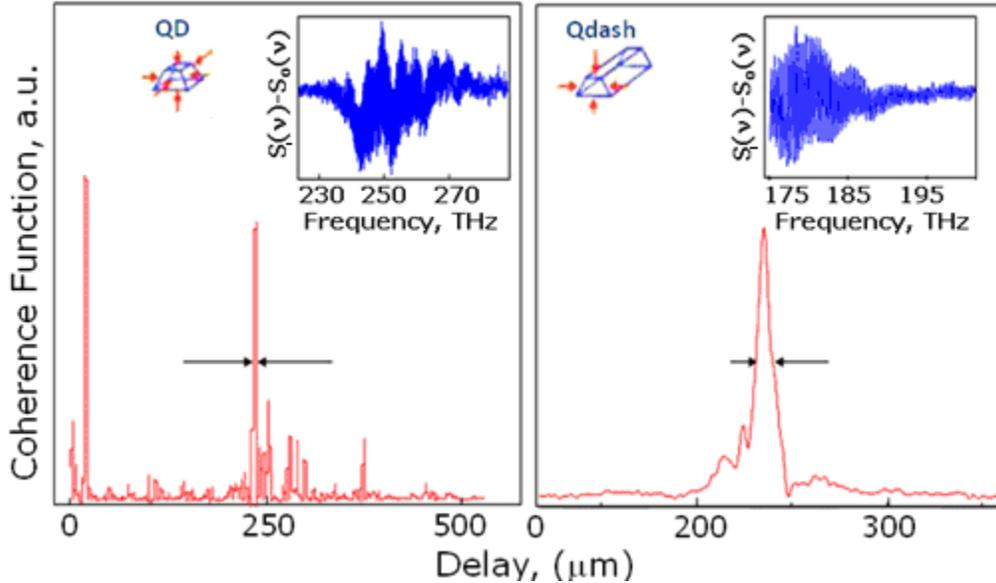
Figure 4. Temporal coherence functions of the InGaAs/GaAs QD (a) and the InAs/InGaAlAs Qdash (b) SLDs taken at 20°C. The insets delineate the intensity of the spectral interferogram minus the input versus frequency.
