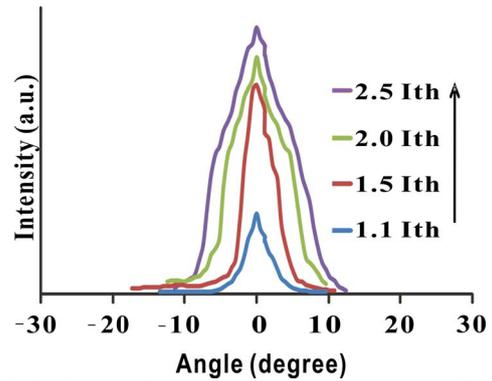
Fig. 2. Far field profiles of the  $50\text{-}\mu\text{m}$ -wide gain-guided Qdash broad area laser with a cavity length of  $0.5 \text{ mm}$  at various current injections.
