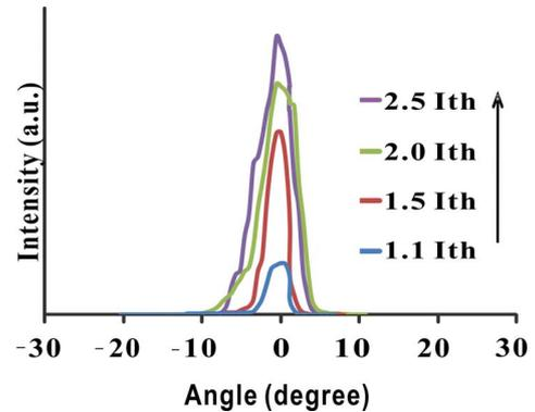
Fig. 3. Far field profiles of the  $50\text{-}\mu\text{m}$ -wide gain-guided Qdot broad area laser with a cavity length of  $1.0 \text{ mm}$  at various current injections.
