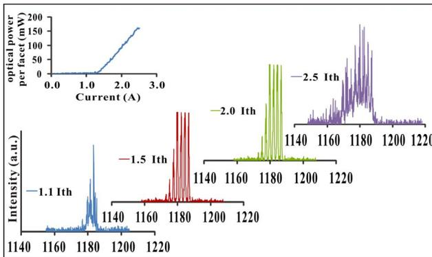
Fig. 6. Electroluminescence spectrum of the 50- $\mu$ m-wide gain-guided Qdot broad area laser with a cavity length of 1.0 mm at various current injections. The inset shows a light-current curve of laser under pulse operation at 15°C.
