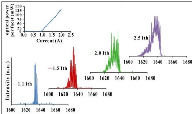
Fig. 5. Electroluminescence spectrum of the 50- $\mu$ m-wide gain-guided Qdash broad area laser with a cavity length of 0.5 mm at various current injections. The inset shows a light-current curve of laser under pulse operation at 15°C.
