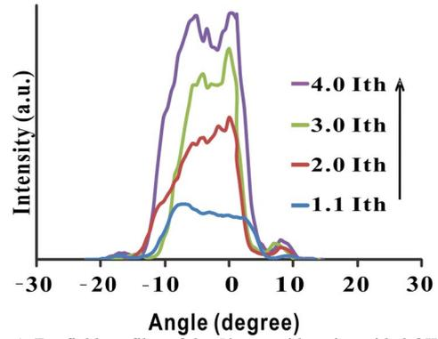
Fig. 1. Far field profiles of the  $50\text{-}\mu\text{m}$ -wide gain-guided QW broad area laser with a cavity length of  $0.5 \text{ mm}$  at various current injections.
