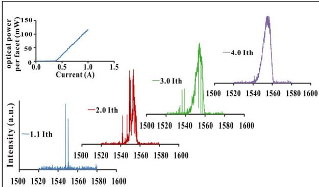
Fig. 4. Electroluminescence spectrum of the 50- $\mu$ m-wide gain-guided QW broad area laser with a cavity length of 0.5 mm at various current injections. The inset shows a light-current curve of laser under pulse operation at 15°C.
