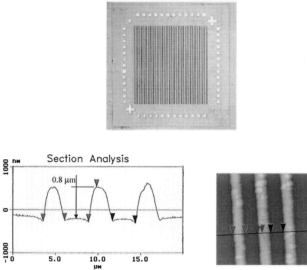
Figure 6. Planarization test chips for developing MEMS interface processes. Top: Micrograph of test chip (4 x 4 mm). Bottom: AFM profile of the passivation layer of the test chip (no via-cut)
