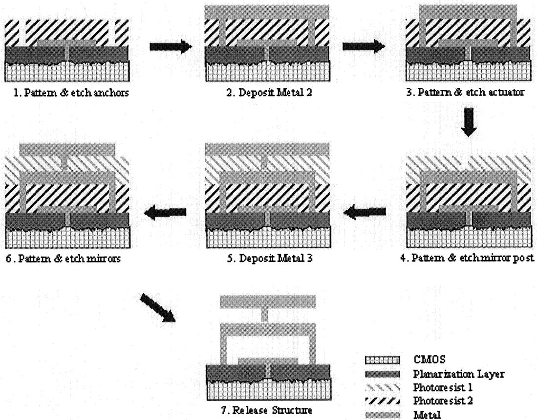
Figure 7b.  $\mu$ SLM actuator and mirror fabrication
