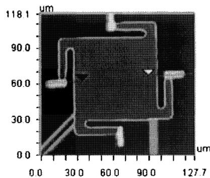
*Figure 8: Interferometric microscope measurement of proof-of-concept metal actuator*
