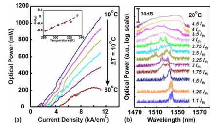
Fig. 2 (a)  $L$ - $I$  characteristics of the  $50 \times 500 \mu\text{m}^2$  broad area Qdash laser at different temperatures. Up to  $\sim 1 \text{ W}$  total output power has been measured at  $J = 5.5 \times J_{\text{th}}$  at  $20^\circ\text{C}$ . (b) The lasing spectra above threshold condition are acquired by an optical spectrum analyzer with resolution of  $0.05 \text{ nm}$ .
