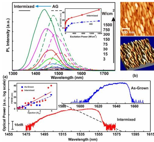
Fig. 1(a) The PL spectra of both AG and intermixed samples with varying optical pumping levels. The inset shows the corresponding changes of FWHM. (b) 2D (top) and 3D (bottom) view of AFM images of InAs QDashes.
