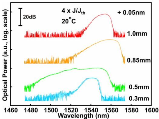
Fig. 4. Effect of cavity dependent on supercontinuum broadband emission from Qdash laser at the injection of  $J = 4 \times J_{th}$ .
