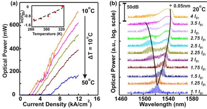
Fig. 1. (a)  $L$ - $I$  characteristics of the  $50 \times 300 \mu\text{m}^2$  broad-area Qdash laser at different temperatures. Up to  $\sim 450$ -mW total output power (from both facets) has been measured at  $J = 4.0 \times J_{\text{th}}$  at  $20^\circ\text{C}$ . (b) Progressive change of lasing spectra above threshold condition.
