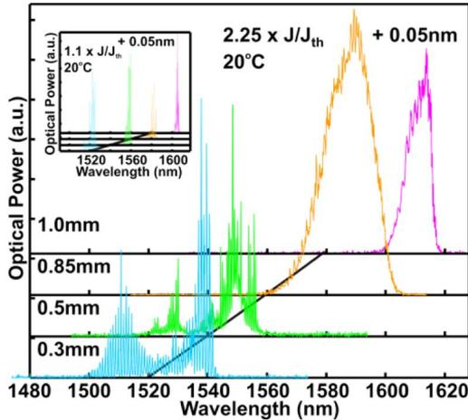
Fig. 3. Presence of different lasing Qdash ensembles with cavity length at the injection of  $J = 2.25 \times J_{th}$ . The inset shows the progressive redshift of lasing peak emission with cavity length at the injection of  $J = 1.1 \times J_{th}$ .
