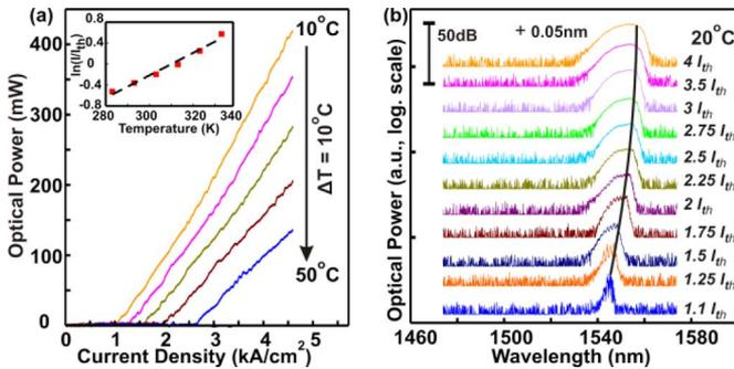
Fig. 2. (a)  $L$ - $I$  characteristics of the  $50 \times 1000 \mu\text{m}^2$  broad-area Qdash laser at different temperatures. Up to  $\sim 340$ -mW total output power (from both facets) has been measured at  $J = 4.0 \times J_{\text{th}}$  at  $20^\circ\text{C}$ . (b) Progressive change of lasing spectra above threshold condition.
