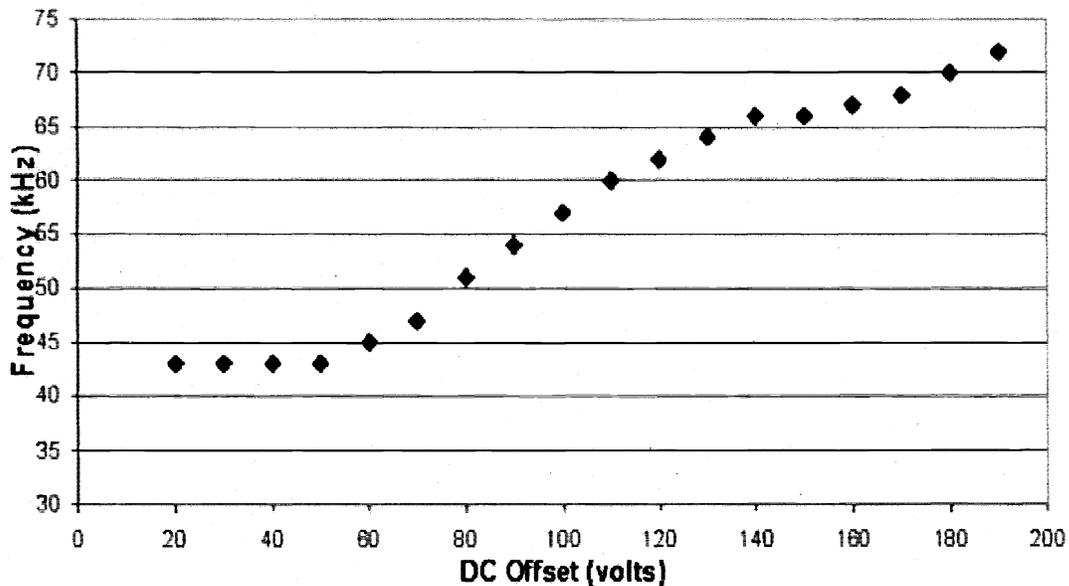
Figure 6. Resonant frequency versus voltage bias at 10 mTorr
