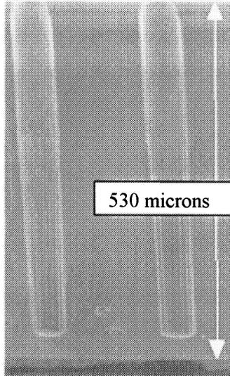
*Figure 7. 50  $\mu\text{m}$  through wafer vias achieving 0.5° or less.*
