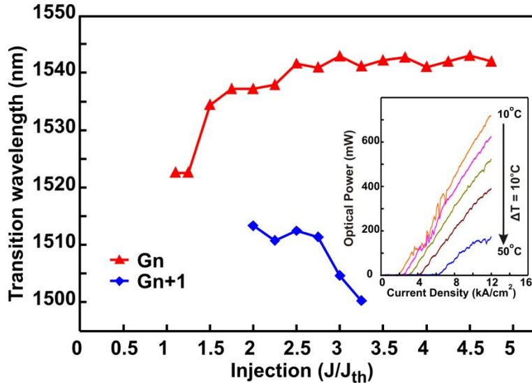
Fig. 2. The progressive change of lasing peak emission from different Qdash ensembles above threshold condition is shown from the  $50 \times 300 \mu\text{m}^2$  broad area Qdash laser. The inset shows the corresponding  $L$ - $I$  characteristics of the laser at different temperatures. Up to  $\sim 450$  mW total output power (from both facets) has been measured at  $J = 4.0 \times J_{th}$  at  $20^\circ\text{C}$ .
