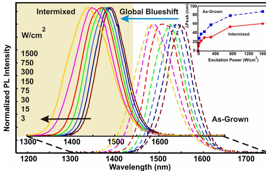
Fig. 1. The PL spectra of both as-grown and intermixed Qdash samples, with varying optical pumping levels, show global blueshift after intermixing. The inset shows the corresponding changes of PL peak wavelength as compared to those obtained under optical excitation of 3  $\text{W}/\text{cm}^2$ .
