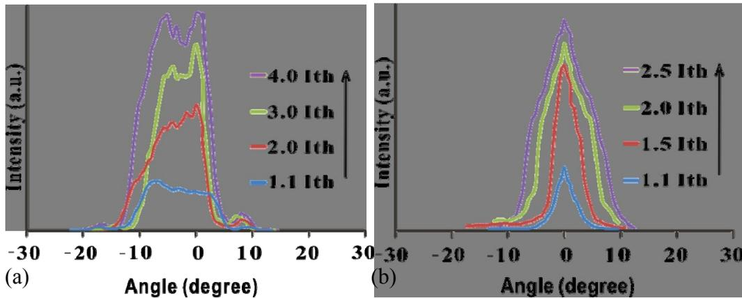
Fig. 4. (a) Far field profiles of the 50- $\mu\text{m}$ -wide gain-guided QW broad area laser with a cavity length of 0.5 mm at different current injections. (b) Far field profiles of the 50- $\mu\text{m}$ -wide gain-guided Qdash broad area laser with a cavity length of 0.5 mm at different current injections.
