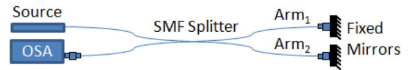
Fig. 1. Schematic of a fiber-based spectral interferometer consisting of a broadband light source coupled into a tapered SMF, a 2 \times 2 fiber splitter, two fixed mirrors, and an OSA for signal detection.
