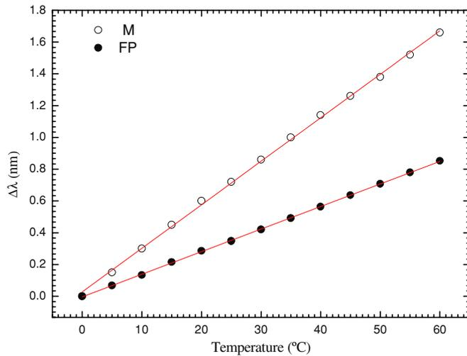
Figure 4. Temperature response for the hybrid interferometer.
