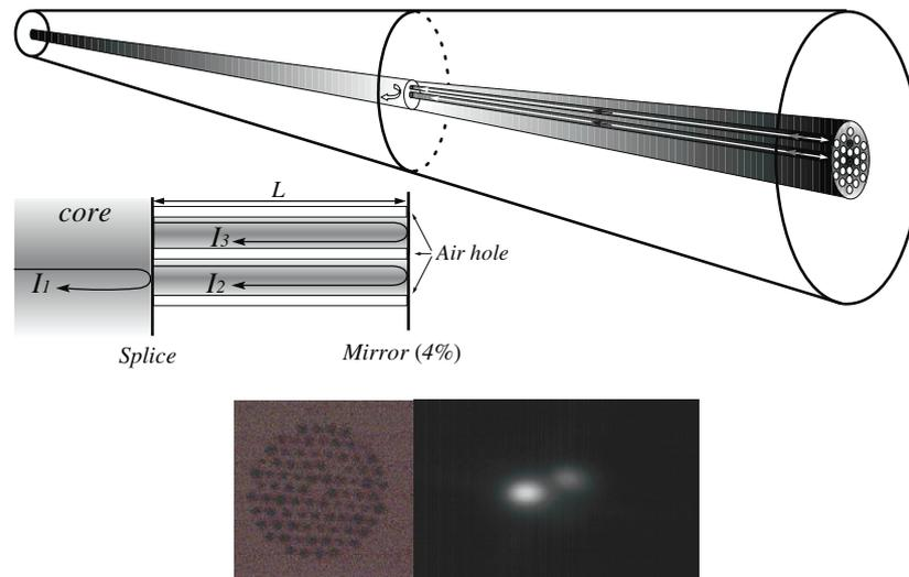
**Figure 1.** (a) Hybrid Fabry–Perot/Michelson interferometer sensor. (b) Cross section of the PCF. (c) Far-field intensity profile (at 1550 nm).
