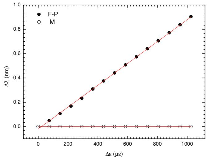
**Figure 3.** Strain response for the hybrid interferometer.
