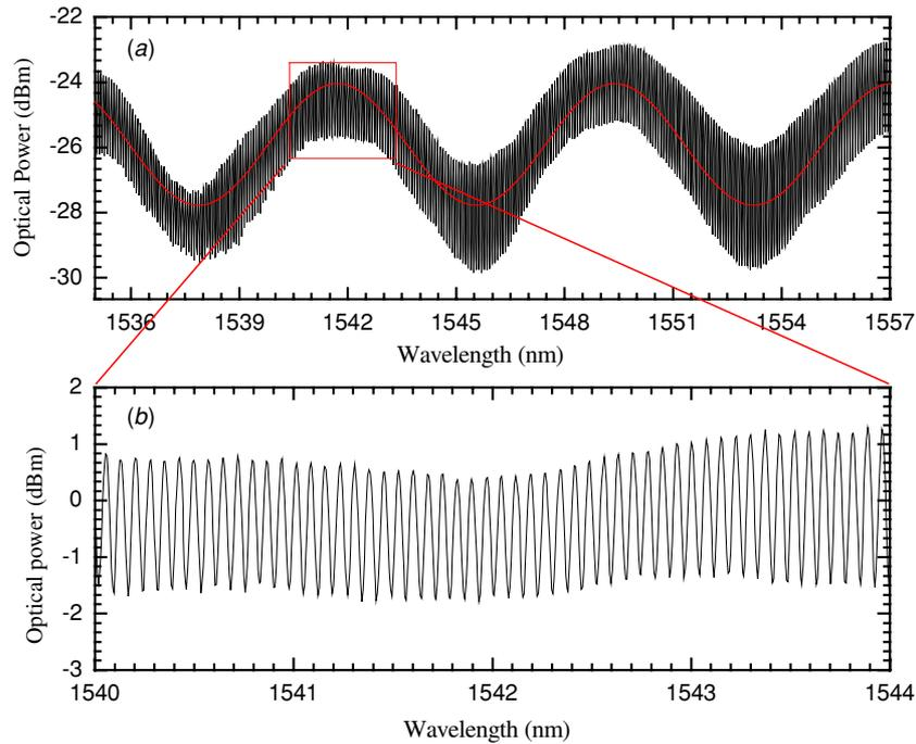
**Figure 2.** Spectral response of the hybrid FP/M interferometer sensor: (a) Michelson and (b) Fabry-Perot.
