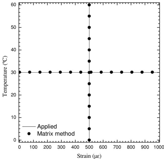
Figure 5. Sensor output as determined by the matrix method for applied temperature and strain.
