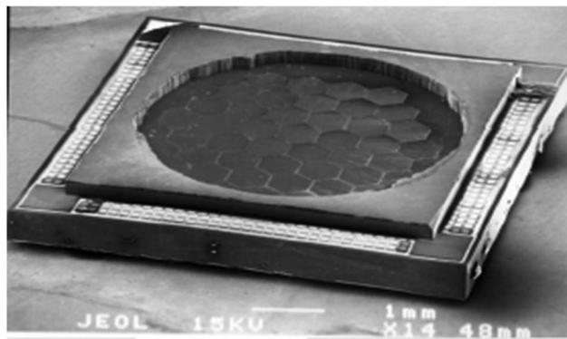
Fig. 3. Iris AO S37-X segmented deformable mirror.
