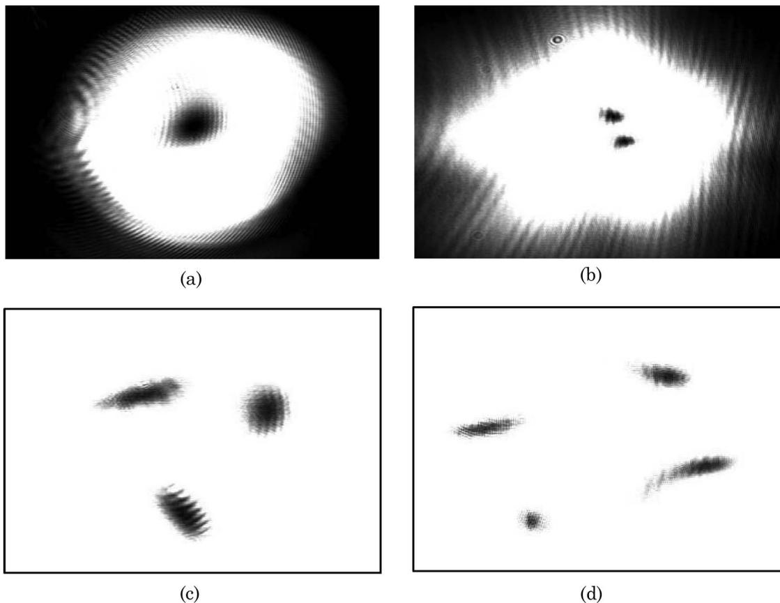
Fig. 5. Decay of multiple-charge optical vortices into charge 1 vortices: (a) charge = 1, (b) charge = 2, (c) charge = 3 (close-up view), (d) charge = 4 (close-up view).
