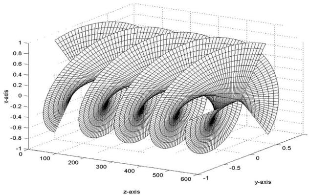
Fig. 1. Wavefront of an optical vortex with charge  $\ell = 3$  (arbitrary spatial units).
