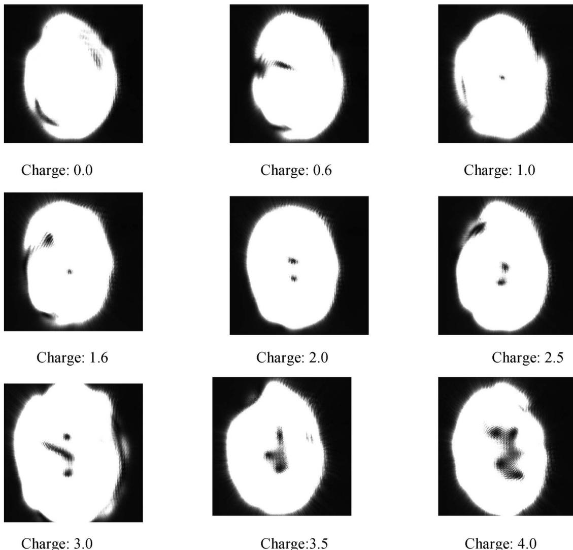
Fig. 7. Evolution of the intensity pattern for the beam reflected off the deformable mirror from charge 0.0 to charge 4.0 obtained by gradually increasing the phase discontinuity.
