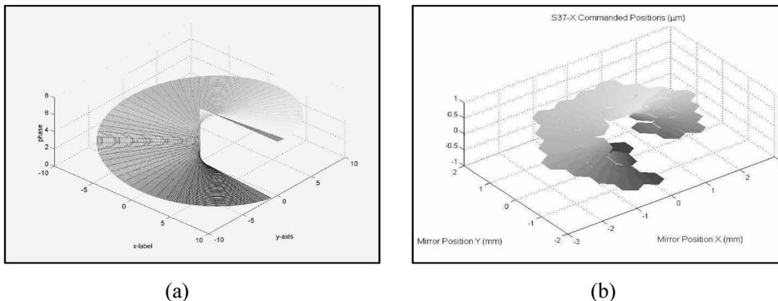
Fig. 4. (a) Ideal linear spiral ramp and (b) ramp approximated by Iris AO deformable mirror.
