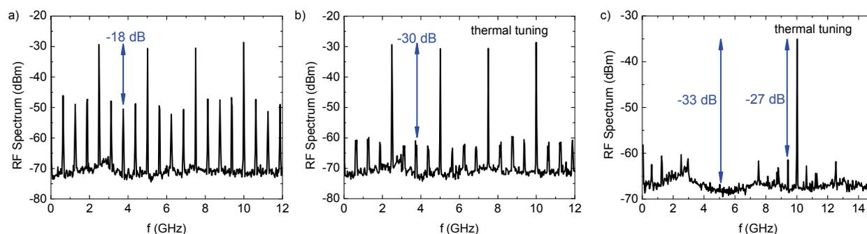
Fig. 3: Comparison of the minimum RF spectrum suppression of subharmonics: a) and b) feature the one-stage interleaver with a 2.5GHz output: thermal tuning reduced the sidebands from  $-18\text{dB}$  to  $-30\text{dB}$ . c) 10GHz pulse train from two cascaded interleaver chips with  $-27\text{dB}$  minimum RF suppression after thermal tuning of the coupling ratios.
