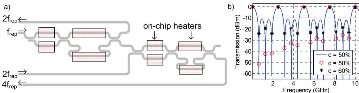
Fig. 1: a) Schematic of the interleaver to quadruple the repetition rate, based on a Mach-Zehnder interferometer with integrated heaters for tuning the coupling ratio and delay line length. b) Simulated transmission for a 2.5GHz interleaver considering the dispersion in the delay lines. The suppression for an ideal coupling ratio of 50% is compared to a coupling of 60% as marked by the red circles and black stars for a 625MHz input.
