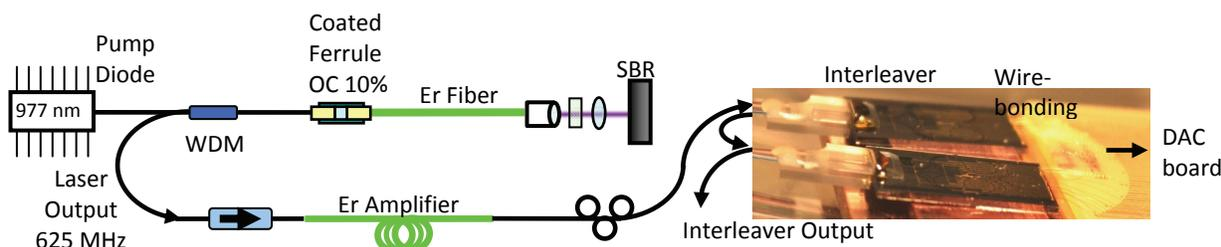
Fig. 2: Schematic of the interleaver system: An erbium-doped (Er) fiber laser is combined with an Er amplifier as the input for the interleaver waveguide chip. One interleaver chip multiplies the repetition rate from 625MHz to 2.5GHz. For a 10GHz pulse train, a second interleaver chip is cascaded after the amplified output of the first interleaver chip. Thermal tuning is performed with heaters controlled by a digital-to-analog convertor (DAC) board.
