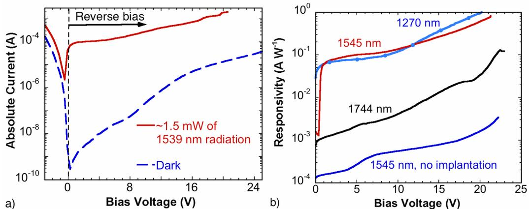
**Figure 11:** Photodiode optical properties. (a) Current-voltage characteristics for a photodiode in the dark and illuminated. (b) Responsivity, which is the ratio of photodiode current to the light entering the diode, for an implanted diode at 1270, 1545 and 1744 nm and an unimplanted diode at 1545 nm.
