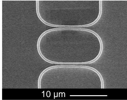
**Figure 8:** Racetrack resonator fabricated in SOI.
