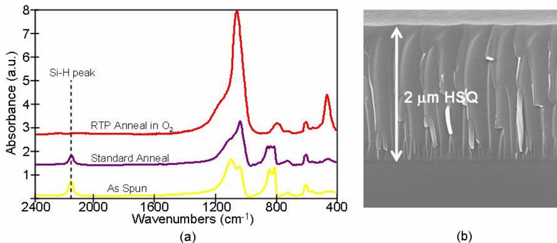
**Figure 6:** (a) FTIR spectra of HSQ as spun, after standard anneal, and after rapid thermal processing (RTP). (b) Cross-section view of 2  $\mu\text{m}$  thick layer of HSQ fabricated using 4 spin coats.
