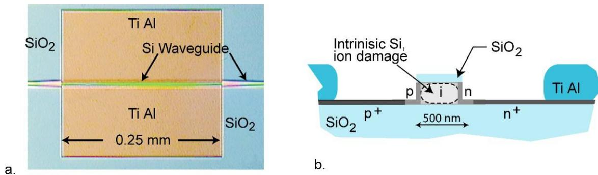
**Figure 10.** Waveguide photodiode. (a) Top-view optical micrograph of 0.25-mm-long waveguide photodiode. (b) Schematic drawing of the p-i-n diode cross section. The waveguide is the intrinsic silicon rib in the center of the sketch.
