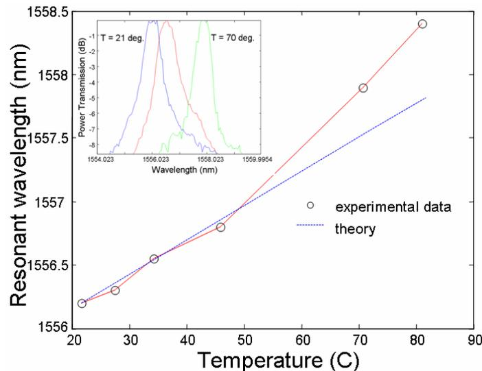
**Figure 7:** Thermal tuning for the second-order filter is observed by changing the temperature of the rings. A total shift of 2.2 nm is observed due to heating the rings from 21°C - 81°C. The inset shows the drop port spectra during tuning.
