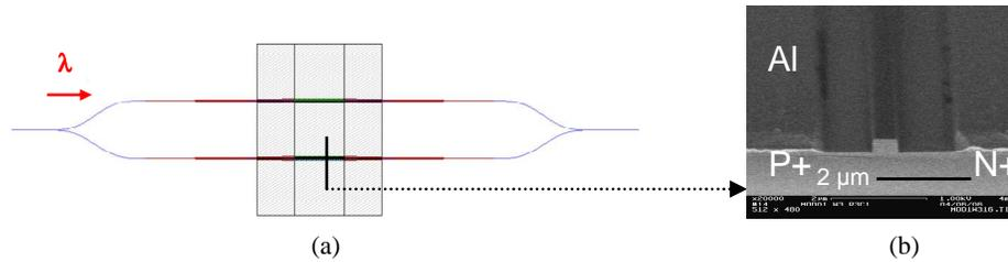
**Figure 3.** Mach-Zehnder modulator. (a) Interferometer shown in plan view. (b) Cross section of diode structure. The silicon rib in the center of the micrograph functions as the optical waveguide and the diode. Current flow through the diode is laterally from the aluminum contacts on the left and right side of the photo. A thin silicon layer connects the metal contacts to the diode. This arrangement isolates the optical mode from the metal contacts and minimizes the optical loss.
